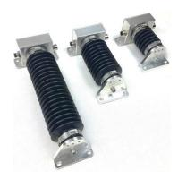
Our displacement sensor may either be used as a standalone unit or as a part of a system together with other daisy chained sensors. In standalone mode the sensor requires 24VDC supply and outputs an analogue current in the range of 4-20mA. The output signal is linearly proportional to the displacement such that 4mA corresponds to 0mm and 20mA represents the maximum displacement of the sensor.
