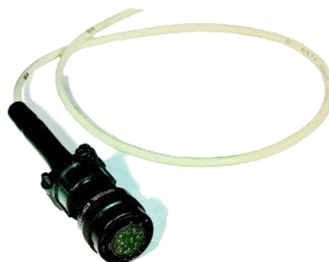
Article no: 01-65103 Cable, PVC, 3m with free soldered ends and socket, MS3116F-12-8S
