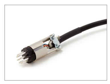
**Note:** Shield should be connected to cable clamp of binder cable assembly when connecting on instrument side. Sensor cable shield connections should be grounded on one end, either the sensor side or the instrument side, to avoid potential ground loops.
